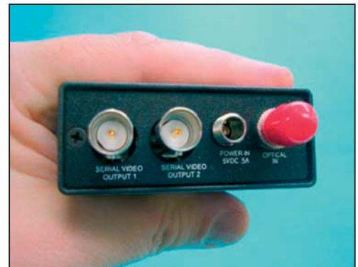
Small, Compact with Re-clocked, Loop-Through Input and Dual Re-clocked Outputs
