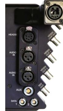
At the rear of the unit are XLR's for Audio MIC inputs 1 and 2 and a 5-pin XLR for Intercom.
