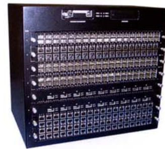
The Multidyne Fiber Optic Switcher can handle 256 x 256 ports
